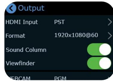
HDMI output defaults multi-screen preview, which can be switched to PGM or the 4 input content in field application.
