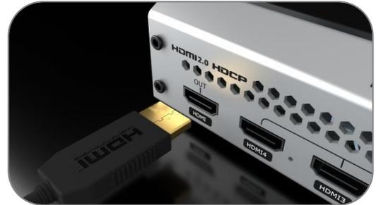
Connect mini-pro HDMI OUT port to monitor to HDMI preview the input and output.
