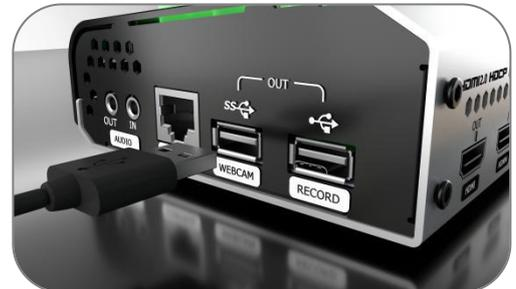
Connect the laptop to mini-pro' s USB 3.0 port via USB cable, and mini-pro will be captured as a webcam source.
