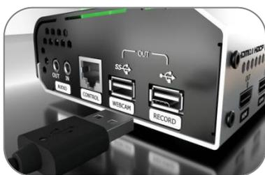
Format the SSD or U-disk and then insert it into the USB2.0 interface RECORD.
