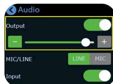
The audio output can be turned on or off, and the volume can be adjusted by sliding the bar.
