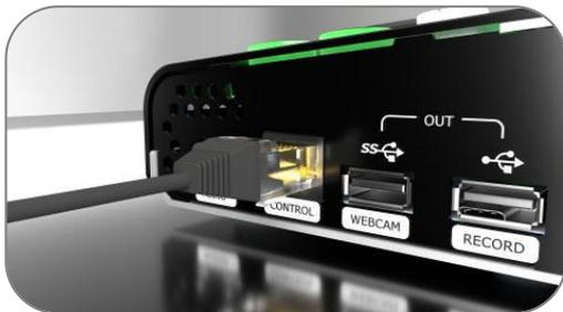
Connect mini-pro' s LAN port to laptop via CAT6 cable, and control mini-pro on software.
