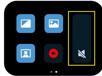
Press button 【 S 】 to enter Shortcut interface, adjust the volume via sliding the bar
