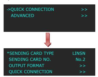
c. Turn the rotary knob, select <SENDING CARD NO.>, push the knob to confirm. Turn the knob and choose "No.1", push the knob to confirm. Shown as follows:
