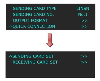
e. Turn the knob, select <RECEIVING CARD SET>, push the knob to confirm. Turn the knob again, and select <CHOOSE CABLE>, push the knob to confirm. Turn the knob, select PORT D1 and push the knob to confirm.
