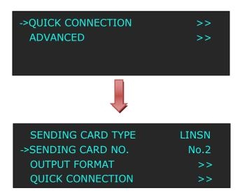
(8) After setting, turn the knob, select <QUICK CONNECTION>, push the knob to confirm for next setting, shown as follows:
