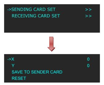
(11) Turn the rotary knob, and select <X>, set X as 360 (Note: X=HORIZONTAL CARD×WIDTH, in the previous part, we set horizontal card as 3 and width as 120). Shown as follows:
