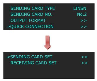
(9) Turn the knob, select <RECEIVING CARD SET>, push the knob to confirm. Turn the knob again, and select <CHOOSE CABLE>, push the knob to confirm. Turn the knob, select PORT U2 and push the knob to confirm.
