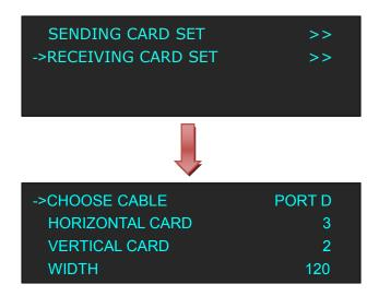
f. Turn the knob, and choose <Offset (A/B) Y>, push the knob to confirm. Turn the knob, set Offset (A/B) Y as 240 (Note: Offset (A/B) Y=VERTICAL CARD×HEIGHT, in the previous part, we set vertical card as 2 and height as 120). Shown as follows:
