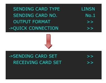
(8) Turn the knob, select <RECEIVING CARD SET>, push the knob to confirm. Turn the knob again, and select <CHOOSE CABLE>, push the knob to confirm. Turn the knob, select PORT U1 and push the knob to confirm.
