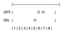
8. Dial switch 5 OFF, dial switch 6, 7 ON: SDI output resolution is 720p 60Hz.
