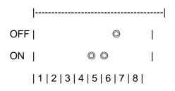
6. Dial switch 5, 7 ON, dial switch 6 OFF: SDI output resolution is 1080i 60Hz.
