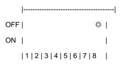
13. Dial switch 8 ON: L-analog and R-analog audio output, no AES/EBU output.
