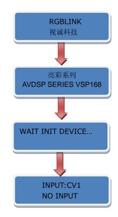
4. After start, the equipment is default load SAVE1 parameter, CV1 key light is on, and the device is in normal working.
