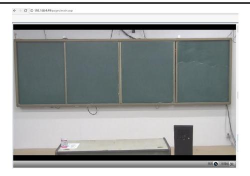
**Platform preset:** Control teacher tracking camera to make platform (we suggest that teachers stand in the middle of platform, if any) get desired visual result in camera image, then click and save platform preset. During normal tracking, size of teacher's image in the picture uses Platform preset as a reference. When tracking target disappears, it can select close-up lens to go back to platform preset.
