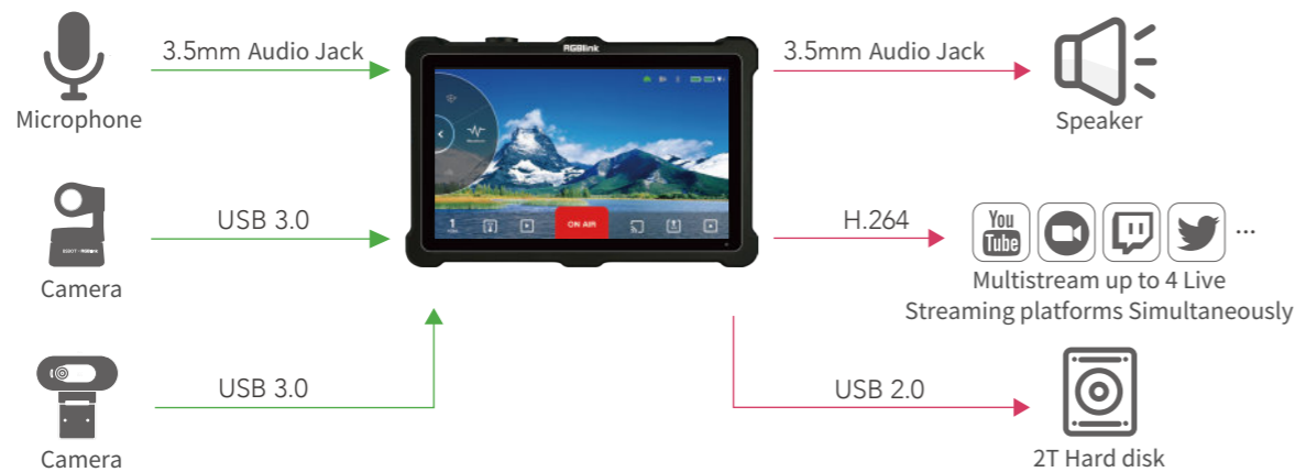
Scene 2: Seamless switching between different USB inputs
