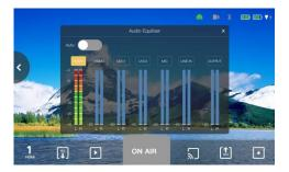
Click Audio Meter to adjust settings of input and output audio.
