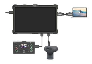
2. Connect the input source to TAO 1pro HDMI IN connector.
