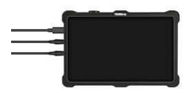
4. Connect microphone to Audio IN interface, speaker or earphones to Audio OUT interface.
