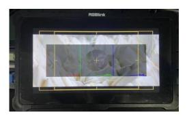
Click [Viewfinder] to select frame size(16:9 or 4:3). Users can cut out the screen outside the frame based on the actual size.
